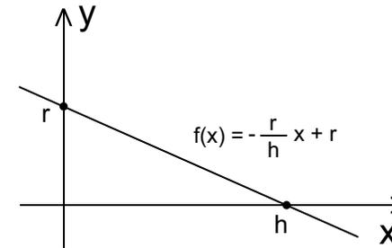
$$V = \pi \cdot \int_0^h \left( -\frac{r}{h}x + r \right)^2 dx = \pi \cdot \int_0^h \left( \frac{r^2}{h^2}x^2 - \frac{2r^2}{h}x + r^2 \right) dx = \pi \cdot \left[ \frac{1}{3} \frac{r^2}{h^2}x^3 - \frac{r^2}{h}x^2 + r^2x \right]_0^h$$
