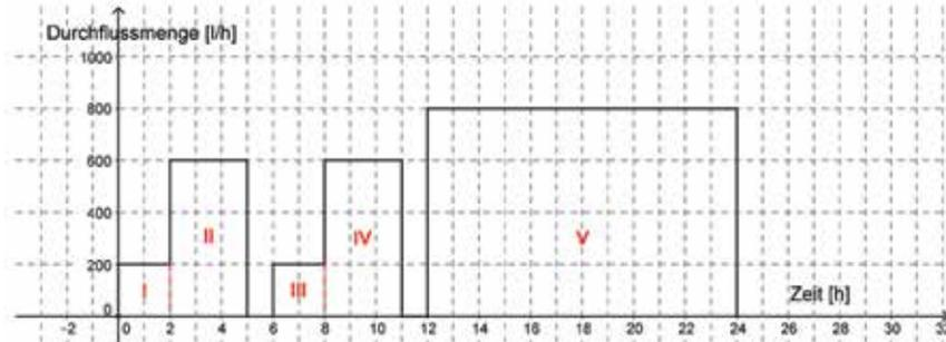
$$A_I = 2 \text{ h} \cdot 200 \text{ l/h} = 400 \text{ l} \quad A_{II} = 3 \text{ h} \cdot 600 \text{ l/h} = 1800 \text{ l}$$
