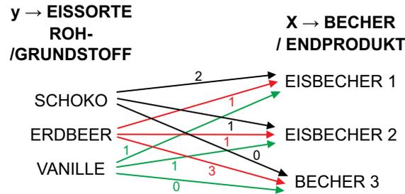
$$\begin{aligned} y_1 &= 2x_1 + 1x_2 + 0x_3 \\ y_2 &= 1x_1 + 1x_2 + 3x_3 \\ y_3 &= 1x_1 + 1x_2 + 0x_3 \end{aligned}$$
